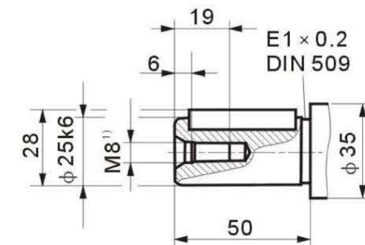
1) centering bore according to DIN 332
