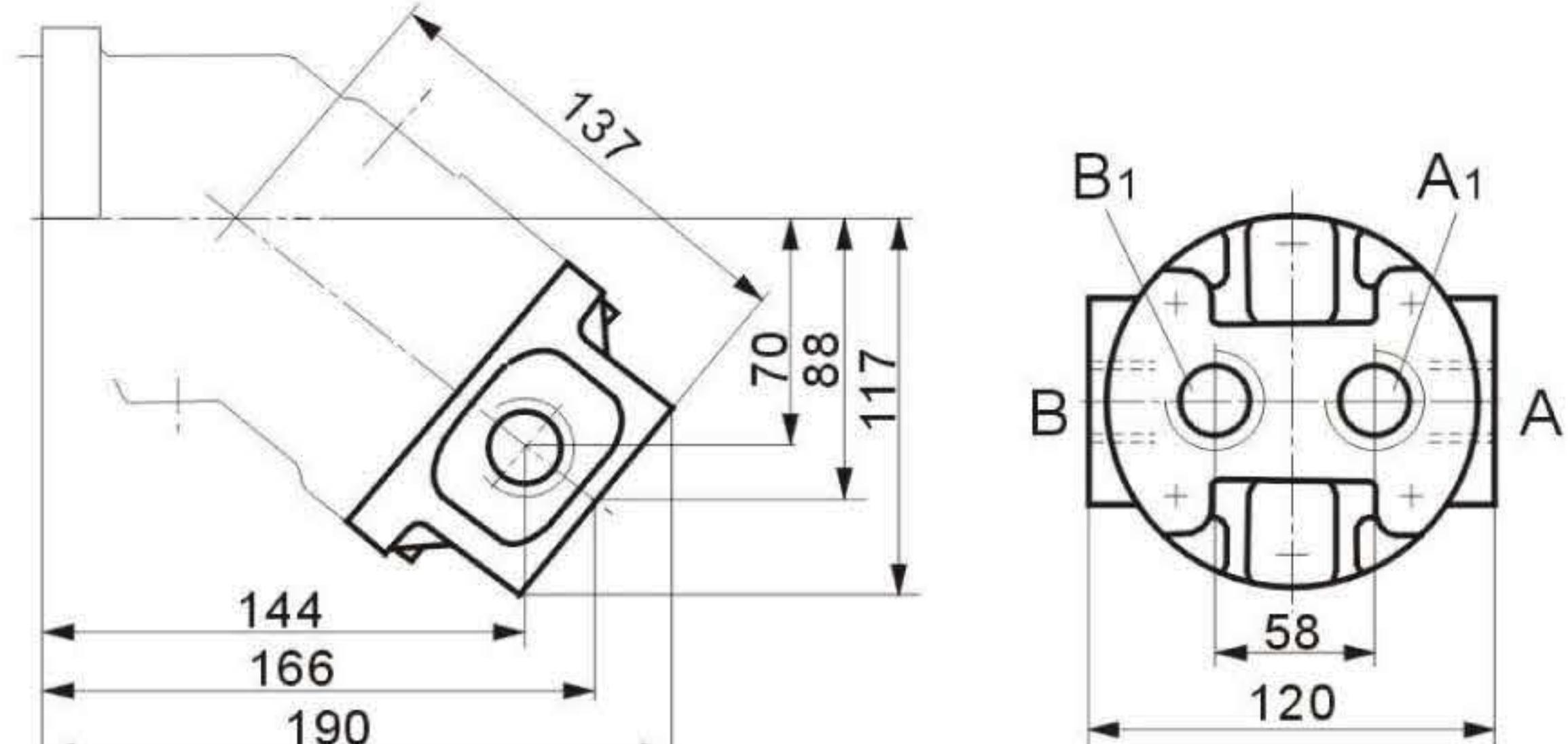
A,B,A<sub>1</sub>,B<sub>1</sub> Service line ports
