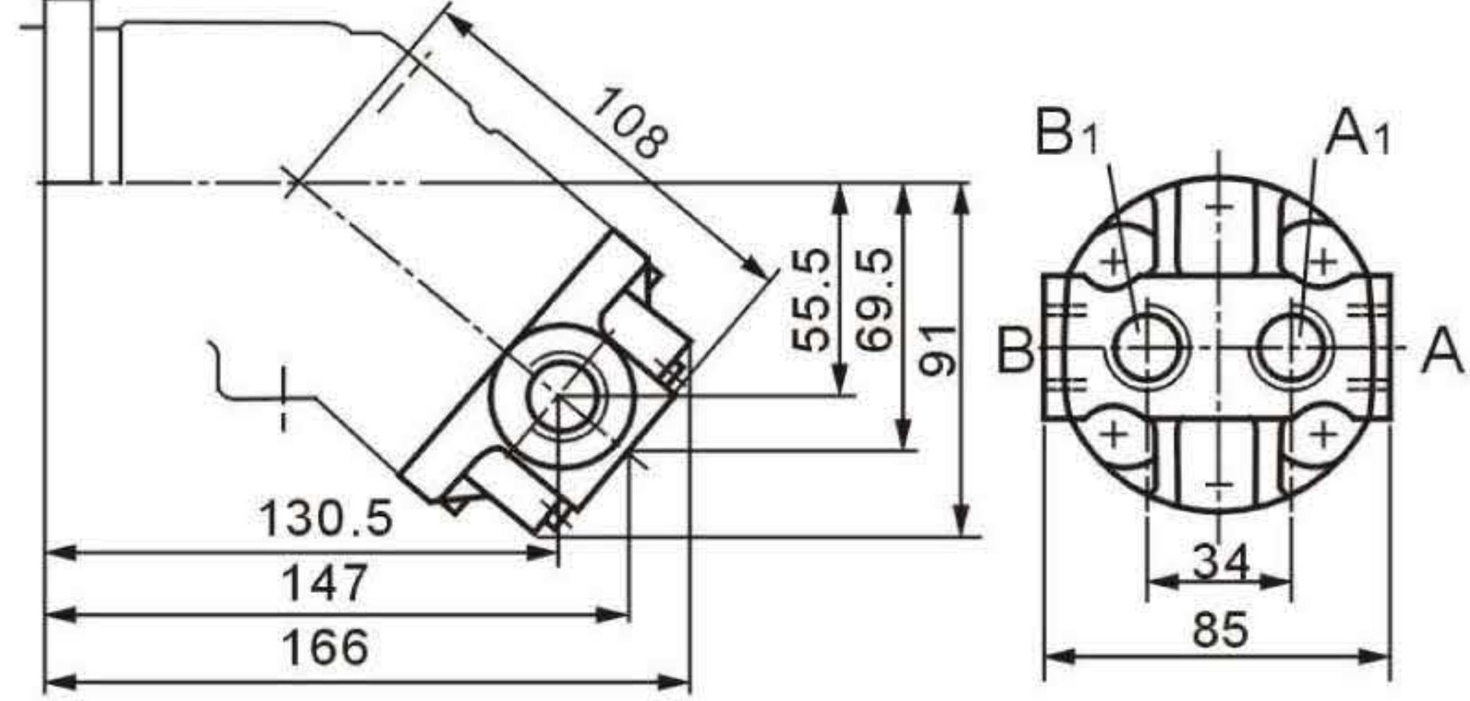
A,B,A<sub>1</sub>,B<sub>1</sub> Service line ports
