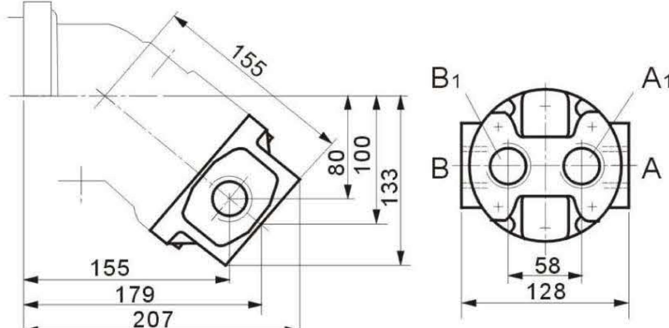
A,B,A<sub>1</sub>,B<sub>1</sub> Service line ports
